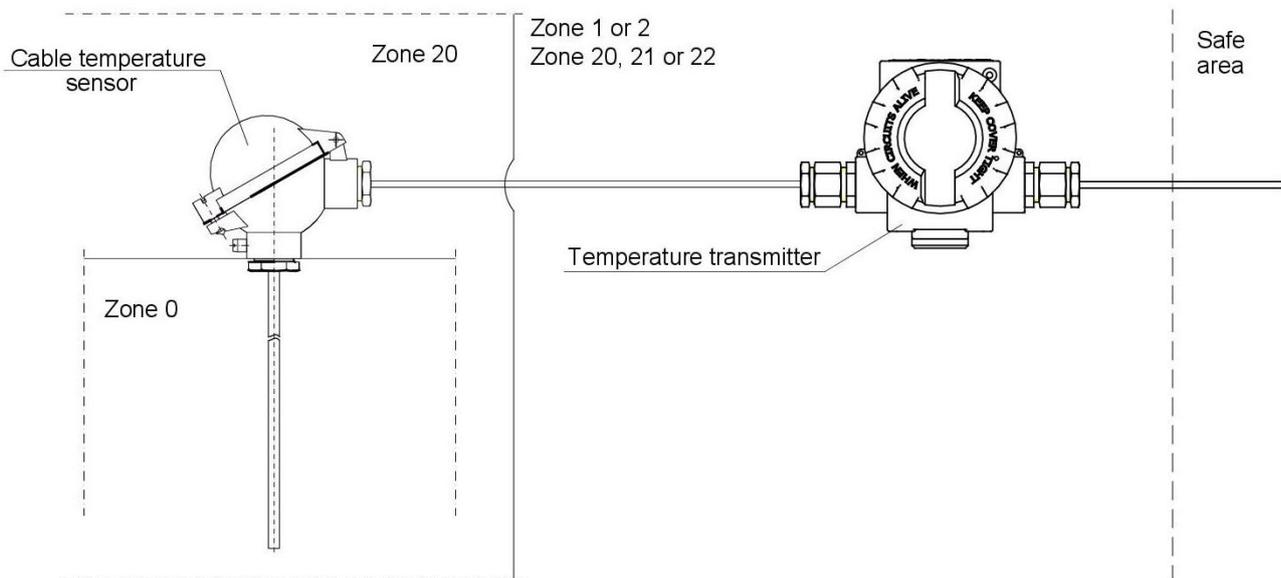
**Figure 1. 3.** LI-24ALW temperature transmitter with a cable temperature sensor.
