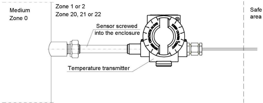
**Figure 1. 4.** LI-24ALW temperature transmitter with a sensor screwed into the enclosure.
