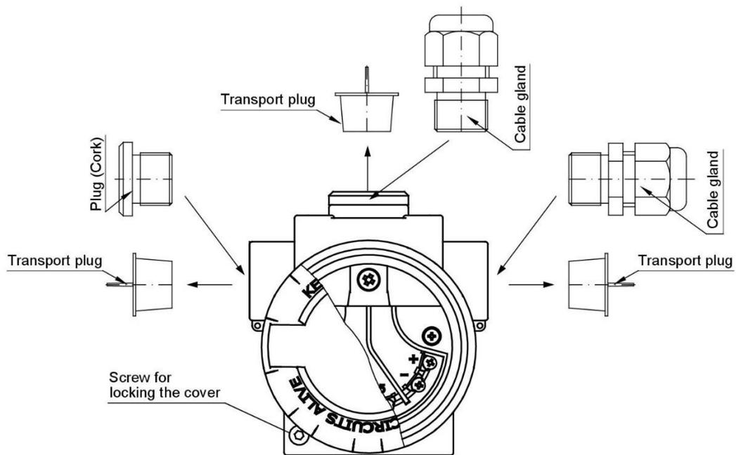
**Figure 1. 10.** Installation of cable entries and blinding plugs (example).
