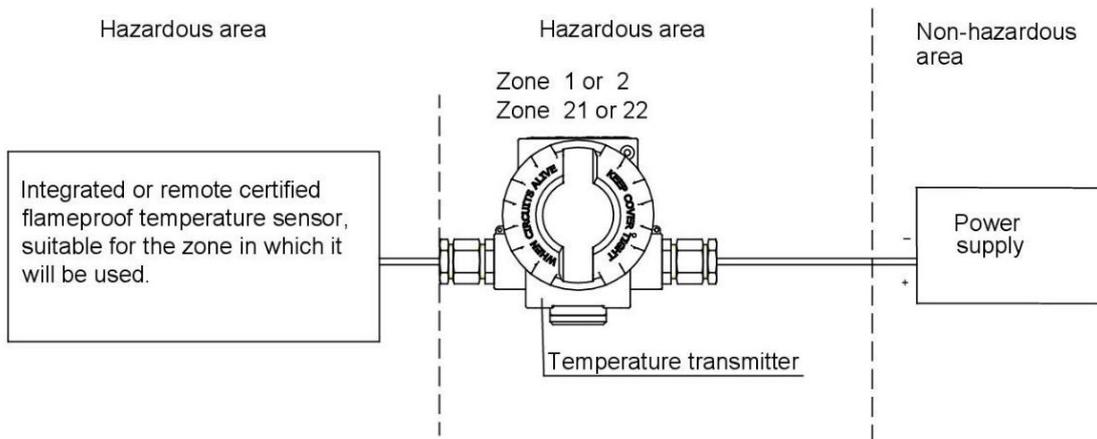
**Figure 2. 5.** Temperature transmitter LI-24ALW Safety with a cable temperature sensor or with a sensor screwed into the enclosure.
