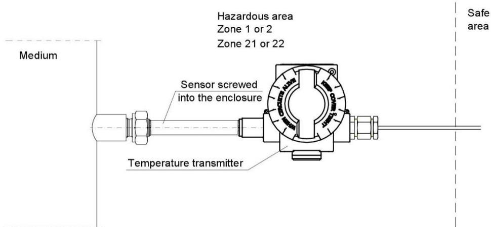
**Figure 2. 4.** LI-24ALW temperature transmitter with a sensor screwed into the enclosure.
