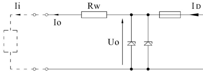
**Figure 1. 6.** The principle of power supply from a source with linear characteristics.
