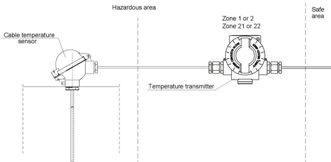
Figure 2. 3. LI-24ALW temperature transmitter with a cable temperature sensor.
