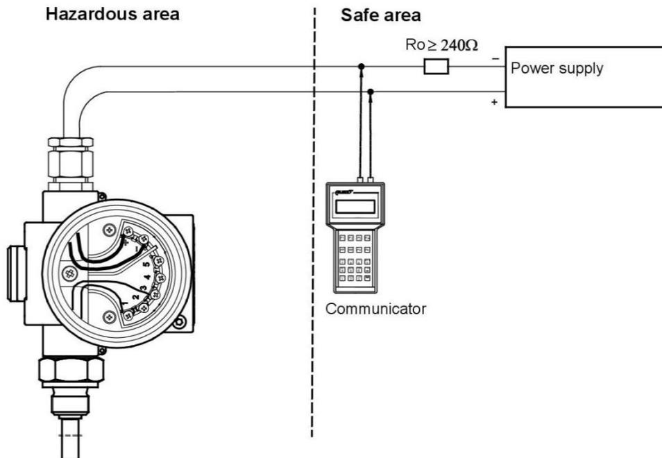
Figure 2. 7. Connection of the transmitter in Exd version.
