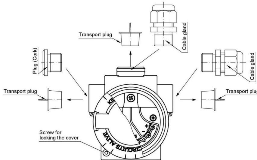
Figure 2. 8. Installation of cable entries and blinding plugs (example).
