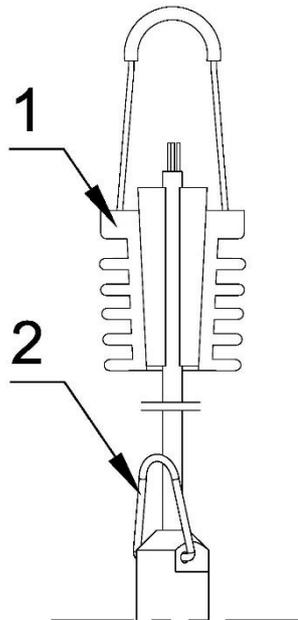
**Figure 2.** Mounting brackets for probes.
