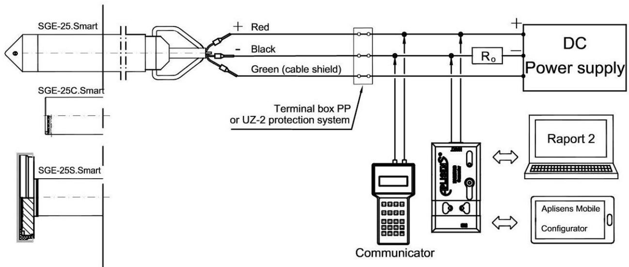
**Figure 4.** Electrical connection 4...20 mA of probes with HART communication.
