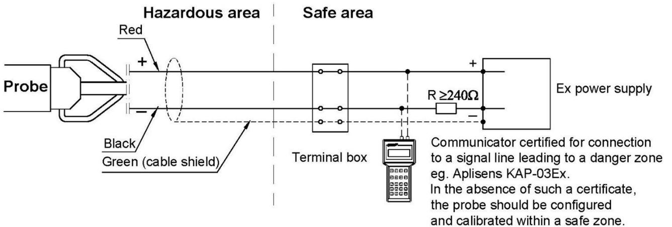
**Figure 1.Ex.** Connection for SGE-25.Smart, SGE-25S.Smart, SGE-25C.Smart probes in Ex version.
