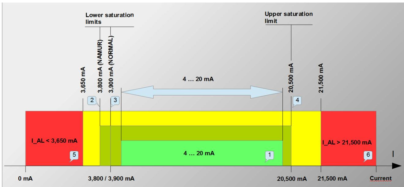
**Figure 5.** Set range current, saturation currents, alarm currents.
