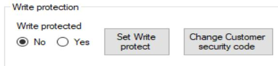
You can set a lock that prevents from modification of the transmitter parameters and change the security code to remove the lock. The lock code has a format of 8 hexadecimal characters, i.e. in the range 0...9, A-F, **the default value is 00000000**. It is not possible to change the transmitter settings when the lock is activated.
