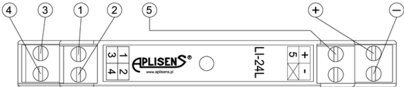
Figure 8. Markings of LI-24L transmitter terminals
